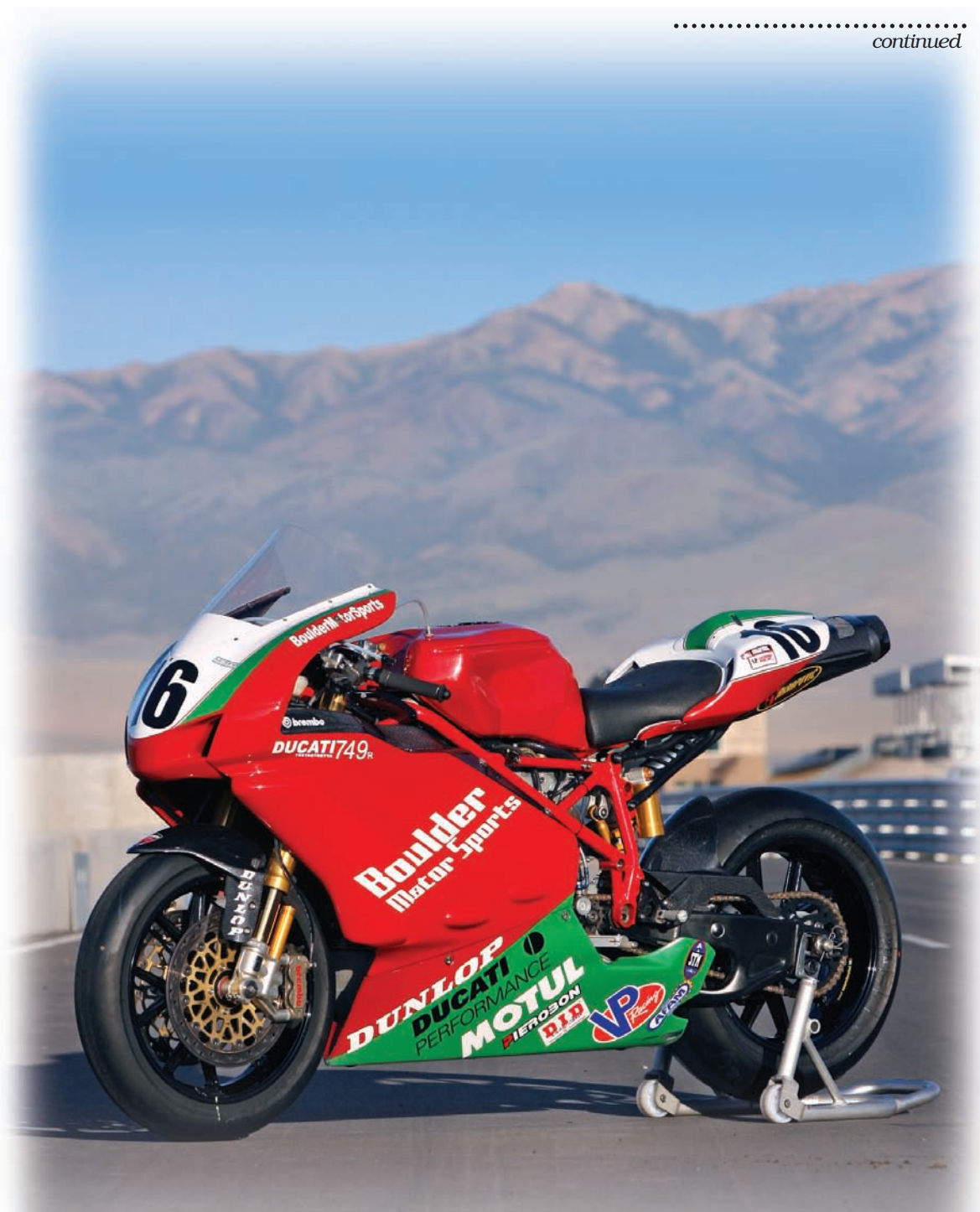
(Opposite page) Chris Ulrich’s first flying lap on the Boulder Motorsports Ducati at Miller Motorsports Park would have been fast enough to qualify for the previous weekend’s AMA Formula Xtreme race. (Above) A pair of 100mm pistons brings the 749R’s displacement up to 848cc, and raises horsepower on a Dynojet Dyno from about 135 to about 150. Photos by Brian J. Nelson.
